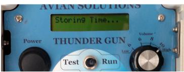
5. To adjust the time of the clock hold the centre switch to test for 5 seconds, scroll the clock to the correct time, then switch to run for 1 second to store the new time.
